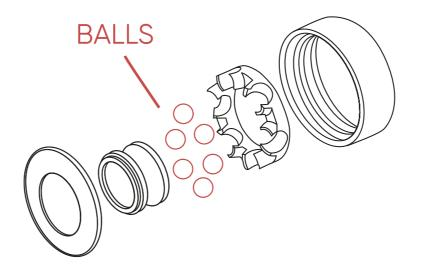
Over the years the materials and technologies available in the bearing industry have progressed significantly. One popular development for bearings was to reduce the number of balls inside the bearing in order to reduce weight and friction. The WCD Twincam ILQ9 pro has 6 balls, compared with its little brother the ILQ7, which has 7 balls, while our Speed Bearing RECORD has 5 balls. It's common to find 7 and 8 ball bearings in the 608 bearing standard.
