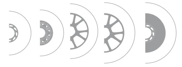
The design of the hub also impacts the wheels performance. If the hub is full like a disc or with lots of spokes it will provide lots of support for the load. The wheel will probably be more reactive and more stable at high speed, but it will also take more vibration.
